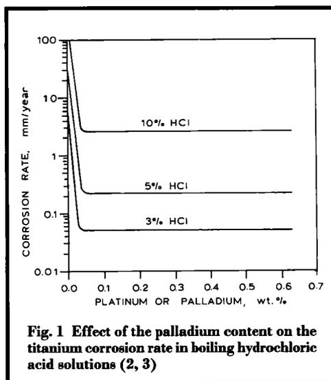
Fig. 1 Effect of the palladium content on the titanium corrosion rate in boiling hydrochloric acid solutions (2, 3)
