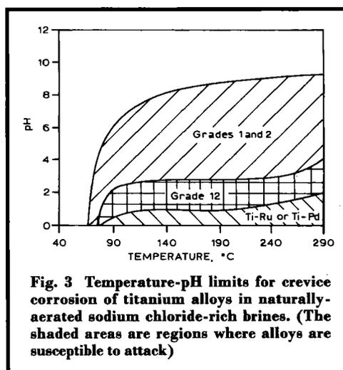
within acidic crevices. The enhanced crevice resistance of Ti-Ru alloys is essentially equivalent to that of Ti-Pd alloys, as indicated by the guidelines in Figure 3.
