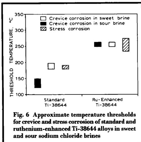
**Fig. 6** Approximate temperature thresholds for crevice and stress corrosion of standard and ruthenium-enhanced Ti-38644 alloys in sweet and sour sodium chloride brines
