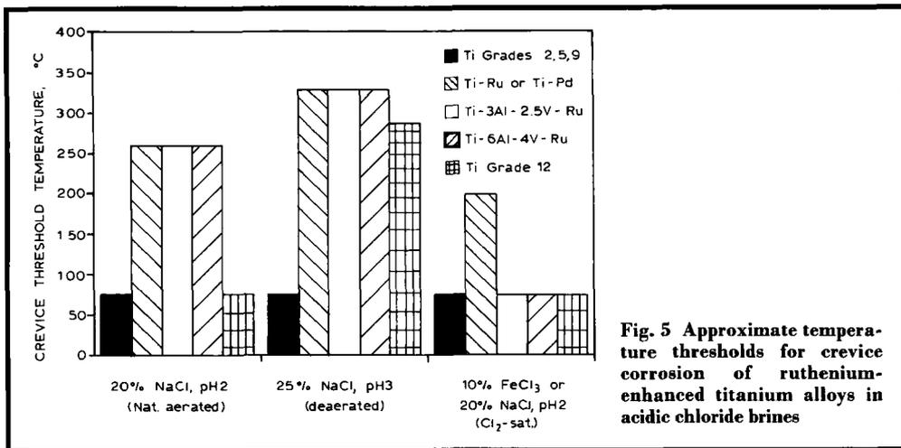
Fig. 5 Approximate temperature thresholds for crevice corrosion of ruthenium-enhanced titanium alloys in acidic chloride brines
