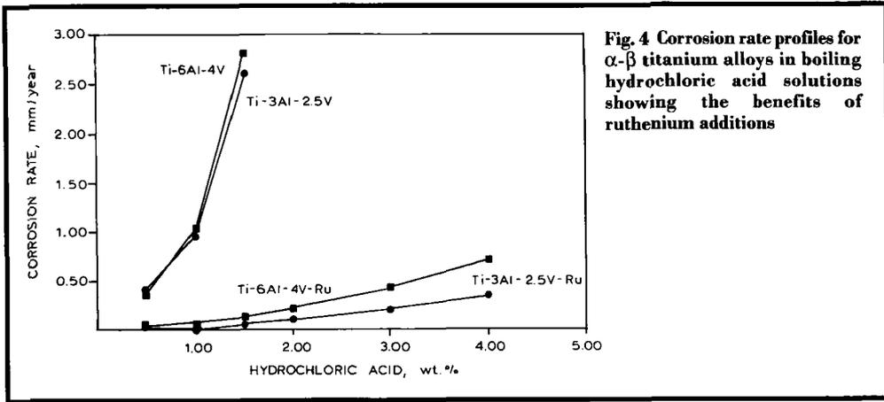
Fig. 4 Corrosion rate profiles for  $\alpha$ - $\beta$  titanium alloys in boiling hydrochloric acid solutions showing the benefits of ruthenium additions
