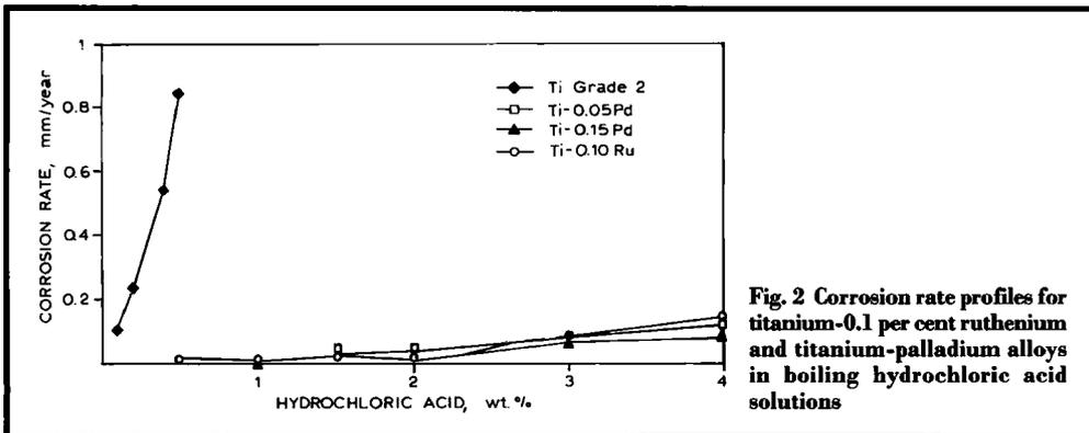
**Fig. 2 Corrosion rate profiles for titanium-0.1 per cent ruthenium and titanium-palladium alloys in boiling hydrochloric acid solutions**
