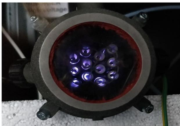
Fig. 6. A catalytic DBD plasma reactor used for the demonstration of CH<sub>4</sub> removal from an engine exhaust
