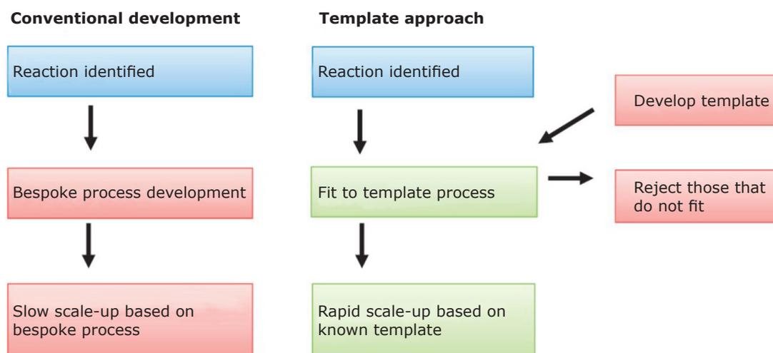
Fig. 3. Concept of template process to accelerate process development. Copyright (2018). Reprinted with permission from Elsevier
