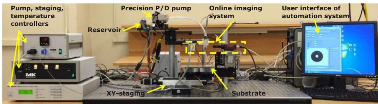
Fig. 2. Dropwise additive manufacturing system. Copyright (2018). Reprinted with permission from Elsevier
