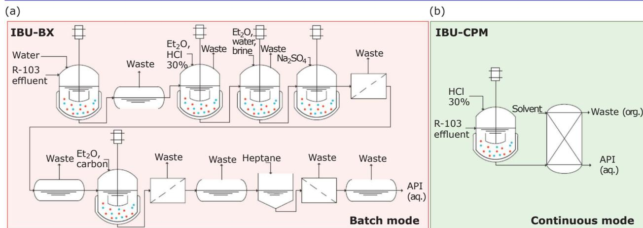
Fig. 4. (a) Batch (2); and (b) conceptual continuous (3, 4) separation schemes for ibuprofen (IBU). Copyright (2018). Reprinted with permission from Elsevier
