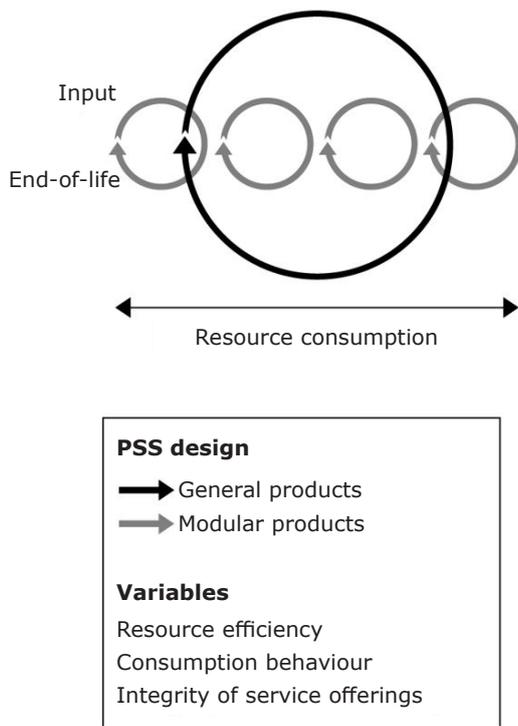
Fig. 4. The misuse of modular design could increase energy or material use
