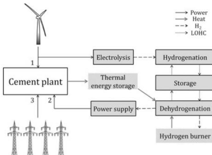
Fig. 3. Schematic representation of the coupling of a cement plant to a LOHC system. Reproduced from Ref. 38, Copyright © 2016 WILEY-VCH Verlag GmbH & Co. KGaA, Weinheim.
