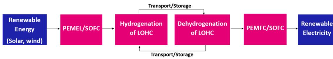
Fig.1. Schematic representation of the integration of fuel cells into LOHC technology.<sup>25</sup>
