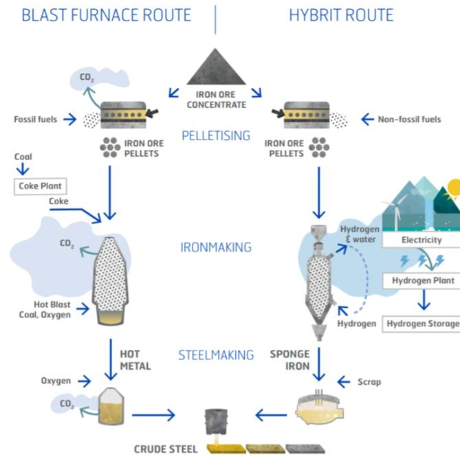
Fig. 4. Steel manufacturing in the HYBRIT route using green hydrogen vs blast furnace route.<sup>46</sup>
