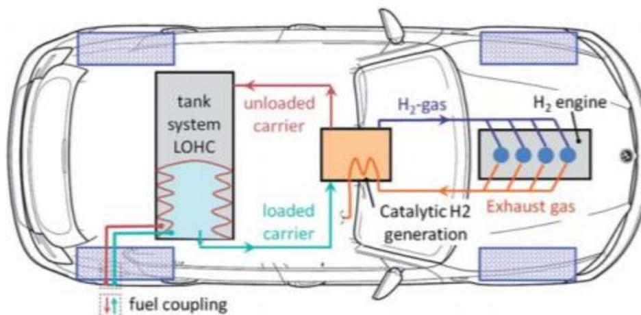
Fig. 5. Schematic representation of the LOHC technology within a motor vehicle.
