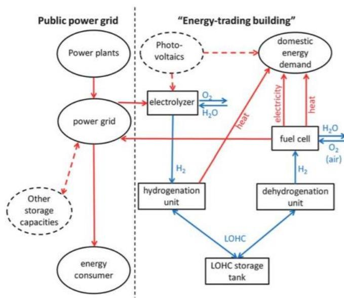
Fig. 2. Concept of integrating LOHC and fuel cell technologies to provide domestic energy. Reproduced from Ref. 34 with permission from The Royal Society of Chemistry.
