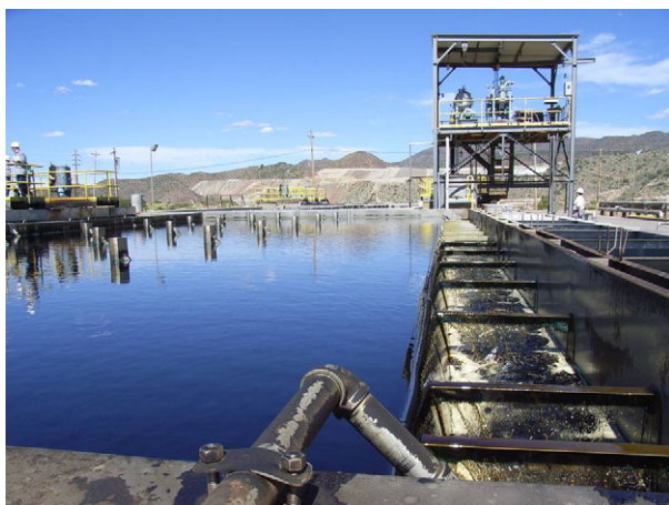
Fig. 2 Typical copper mixer settler as seen on the ISEC post-conference technical tour
