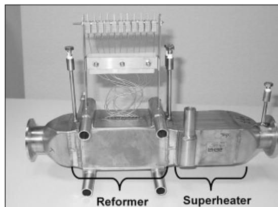
*Fig. 3. Steam reformer with superheater for supplying hydrogen to a PEM fuel cell (Reprinted from M. Grote et al., (7), with permission from Elsevier)*
