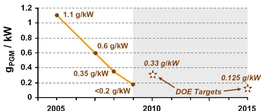
Fig. 6. Status of estimated total pgm content in fuel cell stacks from 2005 to 2009 compared to DOE targets (J. Spendlow, K. Epping Martin and D. Papageorgopoulos, 'Platinum Group Metal Loading', DOE Hydrogen Program Record No. 9018, US Department of Energy, Washington, DC, USA, 23rd March, 2010)
