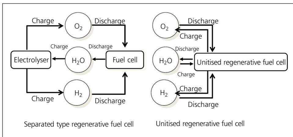
Fig. 5. Schematic of the concept for a 100 W regenerative fuel cell system for use in lunar and planetary missions (Reprinted from Y. Sone, (7), with permission from Elsevier)
