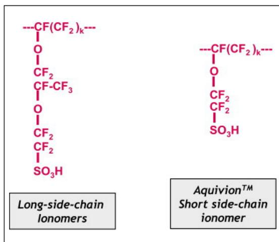
Fig. 7. Polymer structure of long side-chain Nafion<sup>®</sup> and short side chain Aquivion<sup>™</sup> perfluorosulfonic ionomer membranes (Reprinted from A. Stassi *et al.*, (7), with permission from Elsevier)
