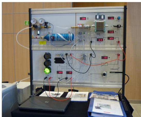
Fig. 2. One of a series of platinum-catalysed fuel cell and solar hydrogen systems for educational purposes designed and built by Heliocentris. This company develops systems and turnkey solutions for training in industry and science, and specialises in hybrid energy storage comprising fuel cells, batteries and energy management devices
