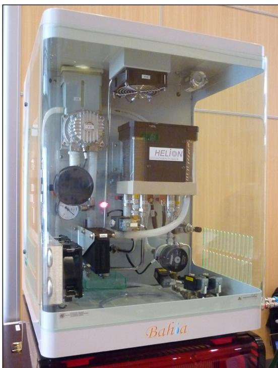
Fig. 1. A 1 kW<sub>e</sub> polymer electrolyte fuel cell and control equipment designed for teaching purposes, exhibited at the Fuel Cells Science and Technology 2010 conference. Operating on pure hydrogen, it can be used to simulate a wide variety of fuel cell and CHP applications. It is built by HÉLION, an AREVA subsidiary, and developed in collaboration with teachers from Institut Universitaire de Technologie (IUT) of Marseille, France
