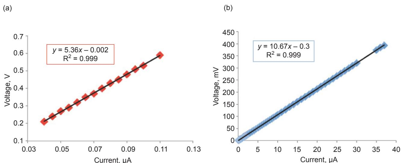
Fig. 5. (a) PtVio V/Volt vs.  $I/\mu\text{A}$  plot; (b) PtAcr V/Volt vs.  $I/\mu\text{A}$  plot. In both cases, the final resistivity values were obtained from the slopes of the linear fits to the experimental points
