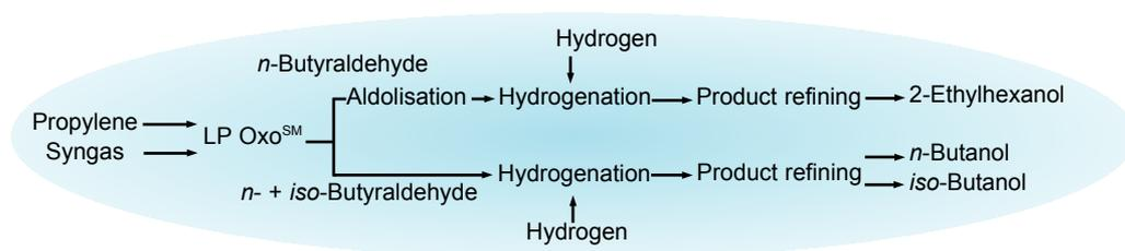
Fig. 1 Schematic showing the production of oxo alcohols from propylene by the LP Oxo<sup>SM</sup> Process
