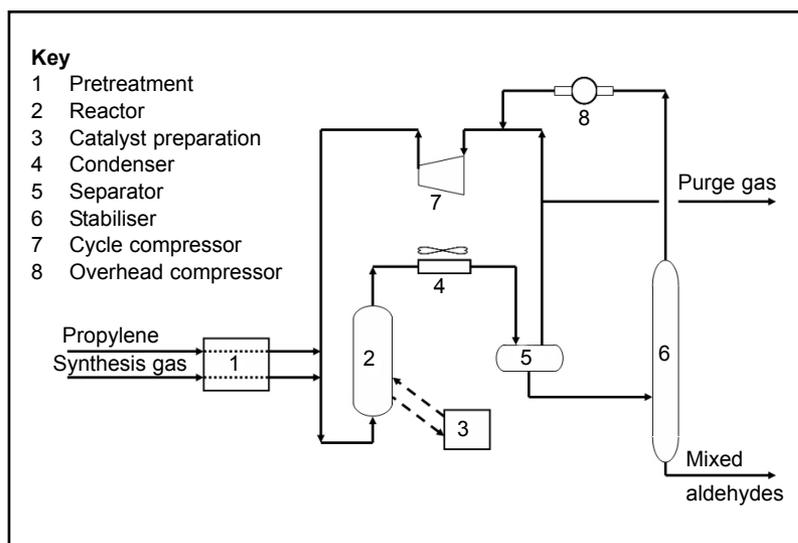
Fig. 3 Gas recycle flowsheet of an early LP Oxo<sup>SM</sup> plant
