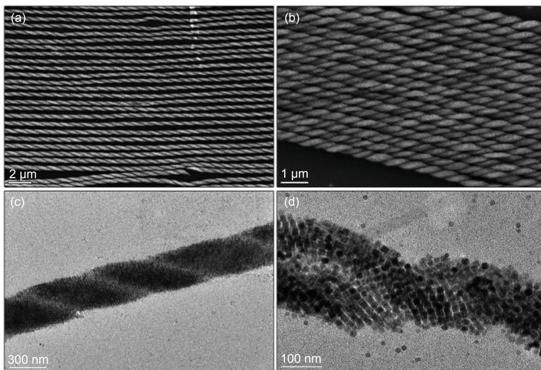
Fig. 2. (a) and (b) Scanning electron micrographs of nanocubes; (c) and (d) transmission electron micrographs showing nanocubes assembled into helical superstructures (4) (Reproduced by permission of The Royal Society of Chemistry)
