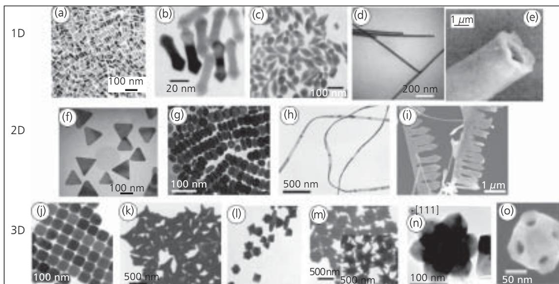
Fig. 1. TEM and SEM images of one-, two- and three-dimensional noble metal nanoparticles: (a) nanorods; (b) nanoshuttles; (c) nanobipyramids; (d) nanowires; (e) a nanotubule; (f) triangular nanoplates; (g) nanodiscs; (h) nanoribbons; (i) nanobelts; (j) nanocubes; (k) nanotetrapods; (l) and (m) star-shaped nanoparticles; (n) a nanohexapod; and (o) a nanocage (Reproduced with permission from Wiley-VCH)
