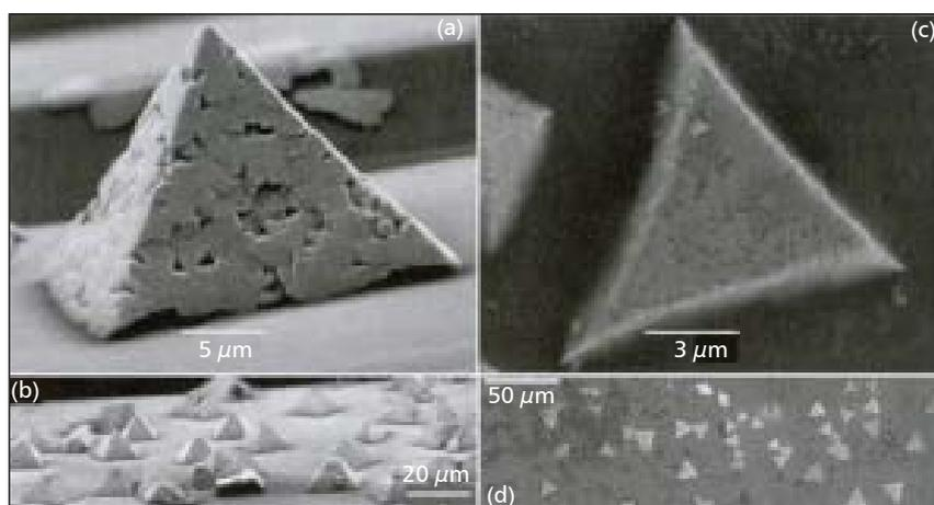
Fig. 2. SEM images of supercrystals of truncated platinum nanocubes: (a) superlattice of pyramidal shape; (b) ensemble of pyramidal supercrystals on a substrate; (c) superlattice of triangular shape; and (d) ensemble of triangular supercrystals on a substrate (Reproduced with permission from Wiley-VCH)
