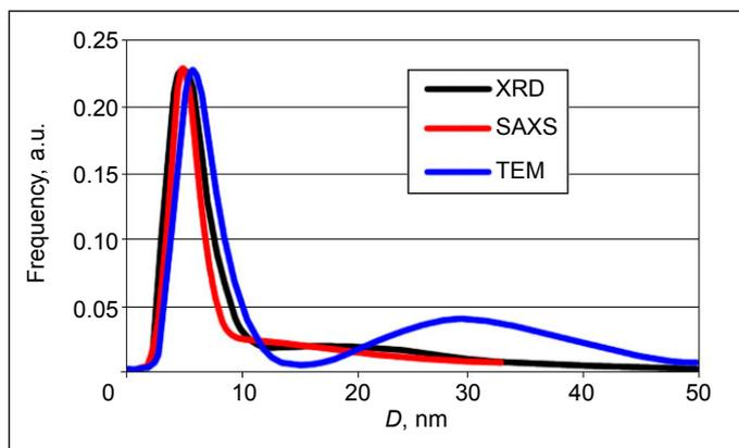
Fig. 2 Comparison of normalised, volume-weighted size distributions determined by XRD, TEM and SAXS for an aged 20 wt.% platinum/carbon electrocatalyst
