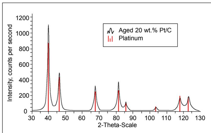
Fig. 1 X-Ray powder diffraction data for an aged 20 wt.% platinum/carbon electrocatalyst
