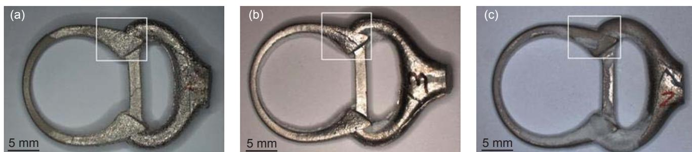
Fig. 7. Macroscopic images showing the surface of as-cast rings of 95% platinum alloys: (a) Pt-5Ru; (b) Pt-1.5Co-3.5Ru; and (c) Pt-5Co
