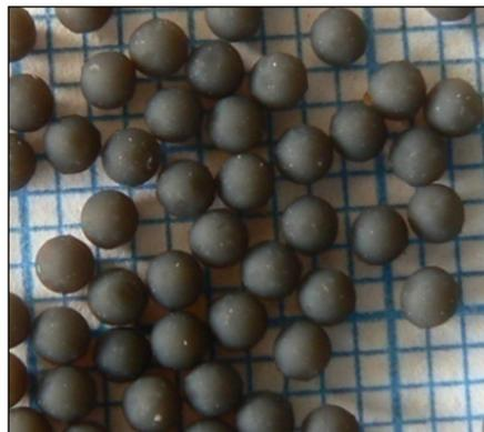
Fig. 2. Black palladium-copper/alginate catalyst for Suzuki coupling (Reprinted with permission from (2). Copyright 2009 American Chemical Society)
