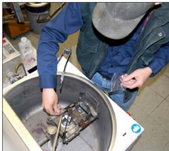
Fig. 1. An induction furnace used for casting platinum jewellery at Au Enterprises, USA. Photograph by Mark B. Mann, Mann Design Group, Inc
