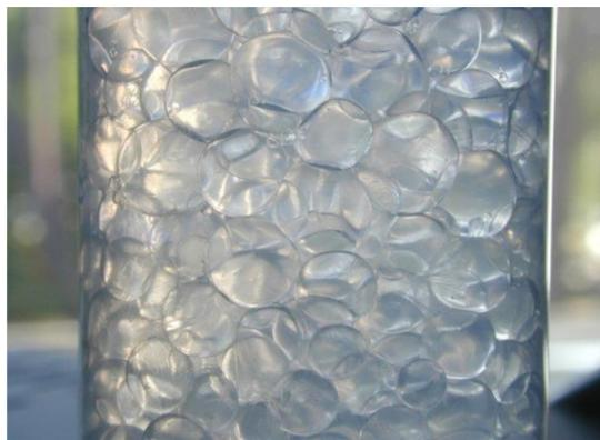
Fig. 1. Oil drops ( $d \approx 1 \mu\text{m}$ ) in water stabilised by 20 nm particles. Reprinted with permission from (1), Copyright (2002), with permission from Elsevier
