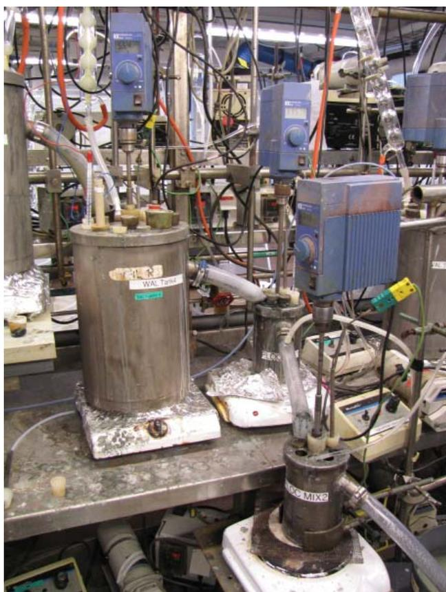
Fig. 1. Rare earth refinery pilot plant leach circuit (Image courtesy of GME Ltd, used with permission)
