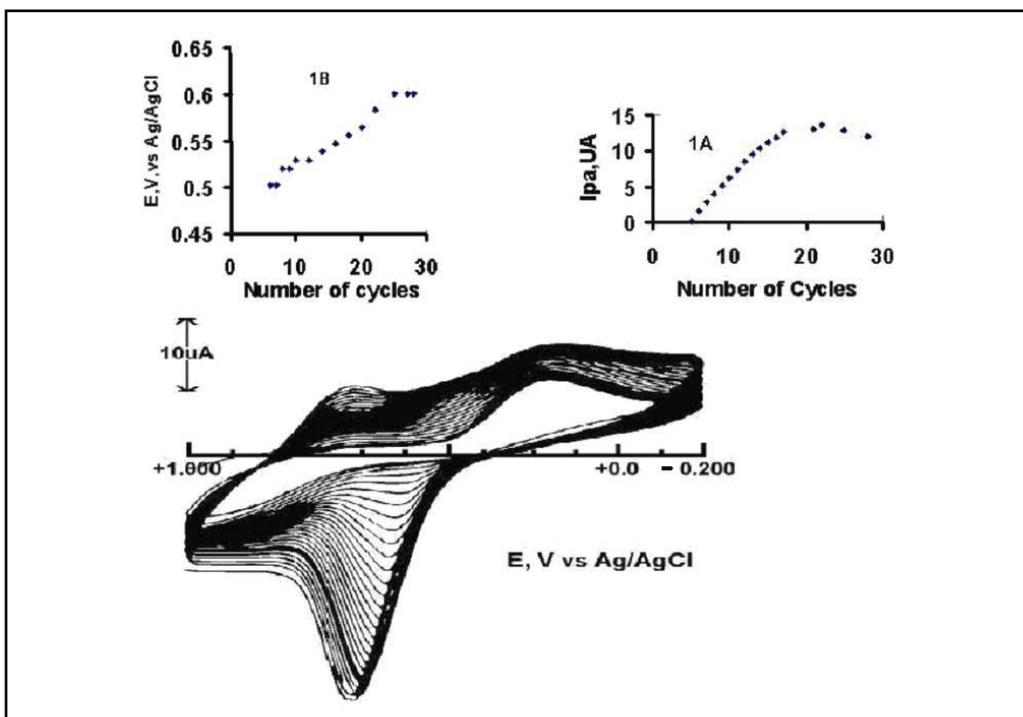
Fig. 1 Repetitive cyclic voltammetry at  $0.1V s^{-1}$  of a glassy carbon electrode (GCE) in equivalent  $1 mM$  of  $K_3[Ir(CN)_6]$  and  $FeCl_3$  in  $50 mM$   $KCl/HCl$  ( $pH = 2$ ). Scan started at  $-0.20 V$  vs.  $Ag/AgCl$
