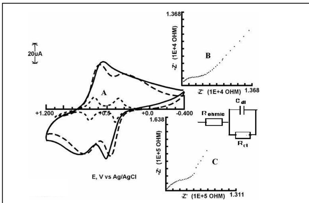
Fig. 4A Cyclic voltammogram of a GCE modified with  $K_xFe_z[Ir(CN)_6]_z$  in 50 mM KCl/HCl at scan rates:  $0.05\text{ V s}^{-1}$  (----);  $0.50\text{ V s}^{-1}$  (-----);  $0.200\text{ V s}^{-1}$  (—)
