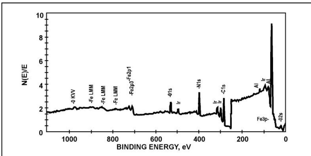
Fig. 3 X-ray photoelectron spectra (XPS) showing the binding energies and intensities of peaks of the aggregates shown in Figure 2
