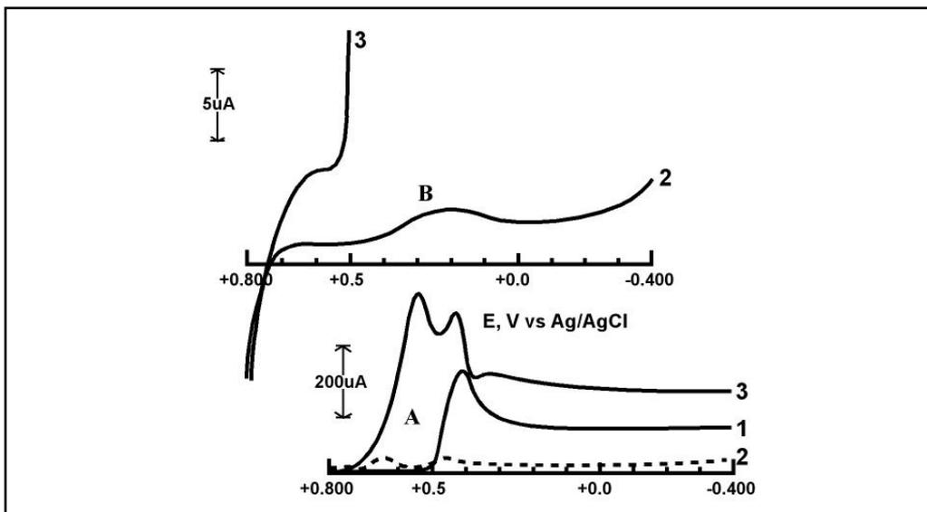
Fig. 7 Electrolytic catalytic activities towards the reduction of  $\text{IO}_3^-$  in aqueous KCl ( $\text{pH} = 1$ ); scan rate  $0.01 \text{ V s}^{-1}$
