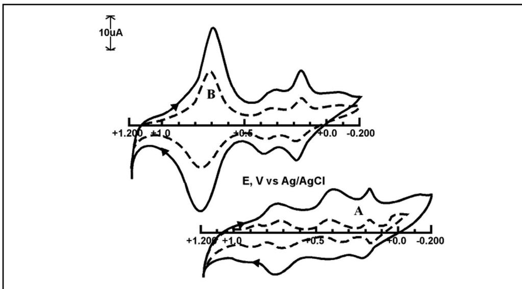
Fig. 6A Cyclic voltammogram of a GCE modified with Prussian blue under  $K_xFe_z[Ir(CN)_6]_z$  in KCl/HCl
