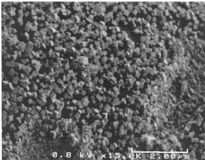
Fig. 2 Scanning electron micrograph of polynuclear hexacyanoiridium(III) films on a GCE surface. The accelerating voltage is 0.8 kV
