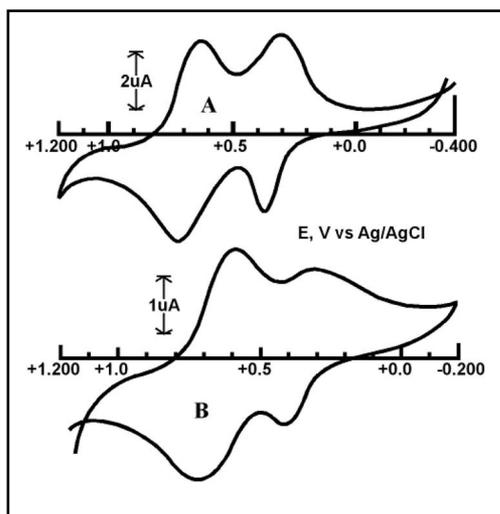
Fig. 5A Cyclic voltammogram at  $0.05 \text{ V s}^{-1}$  of a GCE modified with  $\text{K}_x\text{Fe}_y[\text{Ir}(\text{CN})_6]_z$  in  $50 \text{ mM KCl/HCl}$
