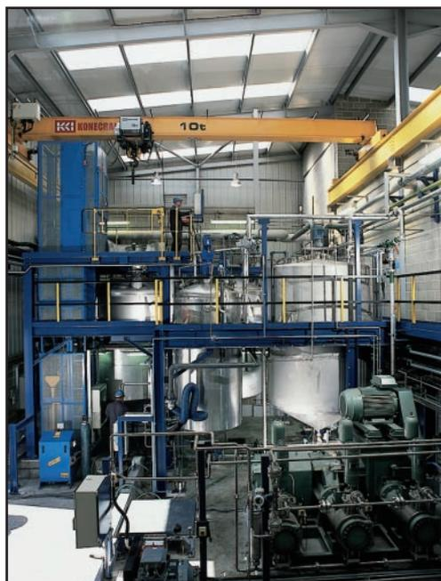
*Fig. 1 Part of AquaCat<sup>®</sup> at the Enfield site. The direct sampling equipment is on the left. The feed tank and high pressure pump for the SCWO process are on the right*
