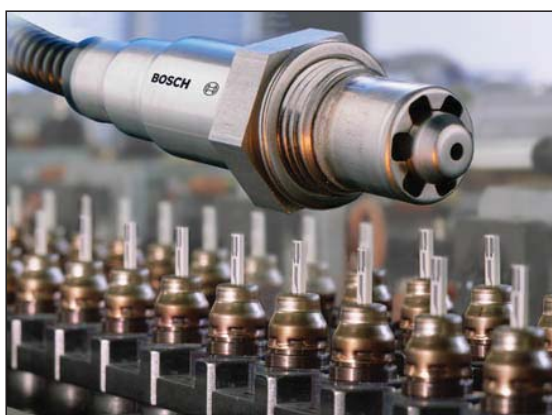
Fig. 8. Oxygen sensors for car exhaust gas (lambda sensors) monitor oxygen levels in the exhaust gases and provide feedback to the electronic engine management system which controls the air to fuel ratio (Copyright © Robert Bosch GmbH)
