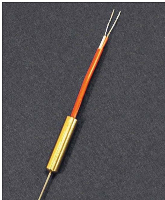
Fig. 9. A thermocouple consists of two wires of different metals joined together at one end to enable the temperature of the joint between the two metals to be calculated
