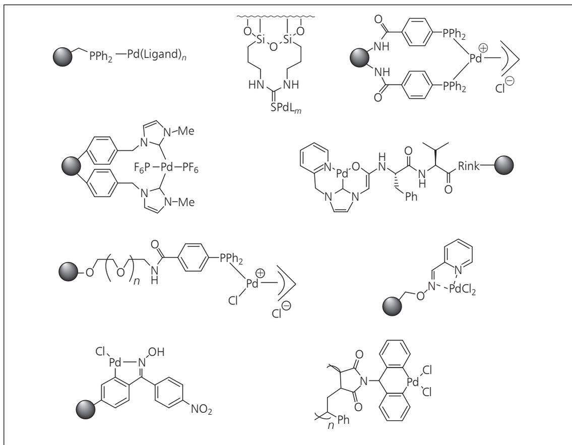
Fig. 3. A selection of polymer-bound palladium catalysts
