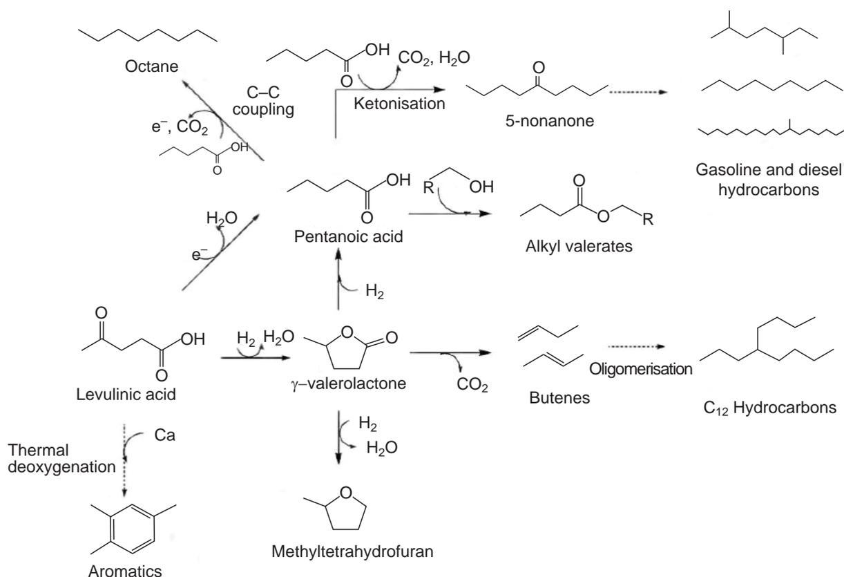
Fig. 1. Scheme of the catalytic routes required to convert biomass-derived acids such as lactic acid and levulinic acid into advanced biofuels
