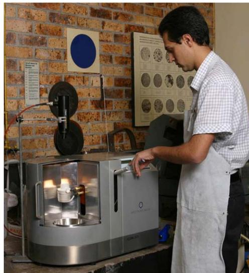
*Fig. 1 Irshad Khan using the Hot Platinum ICON3CS induction melting and casting machine. It can cast up to 250 g of platinum alloy in a single batch*
