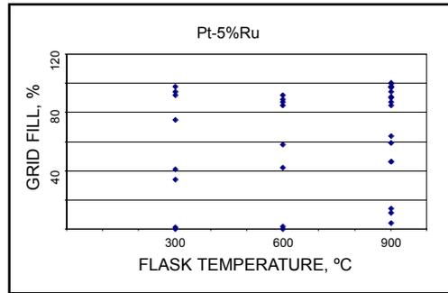
Fig. 5 Plot of percentage grid fill against flask temperature for Pt-5%Ru cast in Platincast investment. No discernable dependence can be seen
