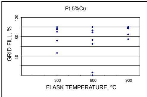
Fig. 3 Plot of percentage grid fill against flask temperature for Pt-5%Cu cast in Platincast investment. No discernable dependence can be seen
