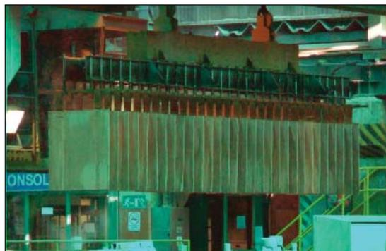
Fig. 4. Copper cathodes in copper electrowinning plant in Chile (Image copyright Emma Schofield, Johnson Matthey Technology Centre, UK)
