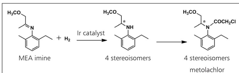
Fig. 3. A process for the preparation of (*S*)-metolachlor
