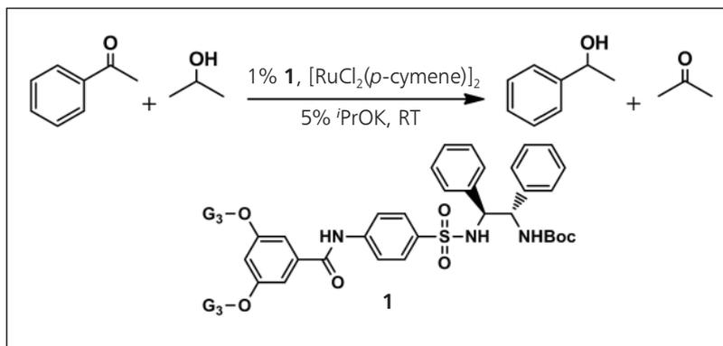
Fig. 2. Asymmetric transfer hydrogenation with ruthenium on dendrimer catalyst.  $G_3$  = generation 3 dendrimer
