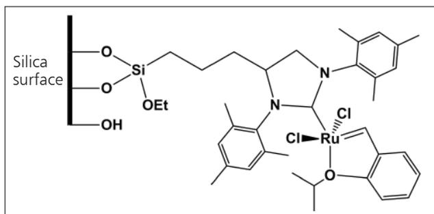
Fig. 5. Heterogenisation of Grubbs olefin metathesis ruthenium catalyst
