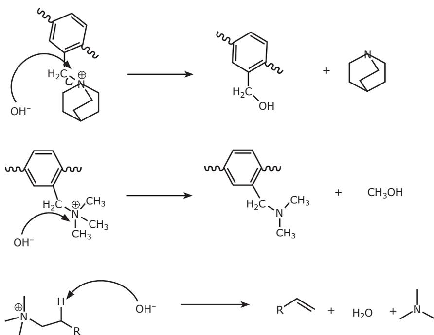
Fig. 1. Degradation mechanism for quaternary ammonium-based anion exchange membranes
