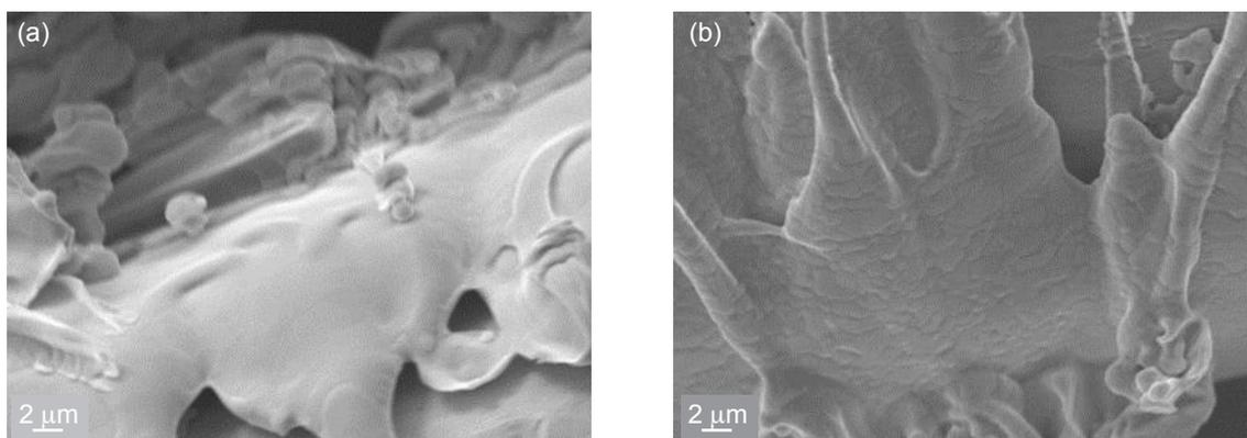
Fig. 11. SEM images of the ACT™ coating: (a) before and (b) after restructuring
