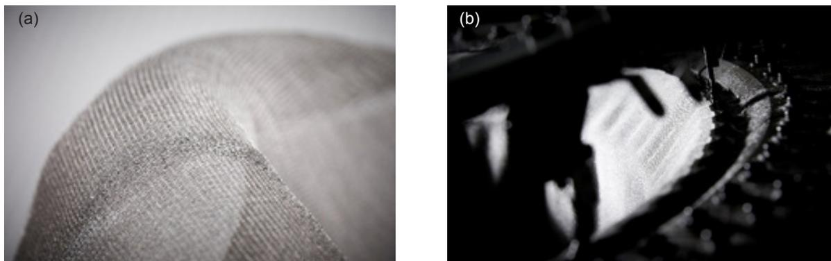
Fig. 2. (a) The structure of a knitted gauze; (b) a gauze knitting machine
