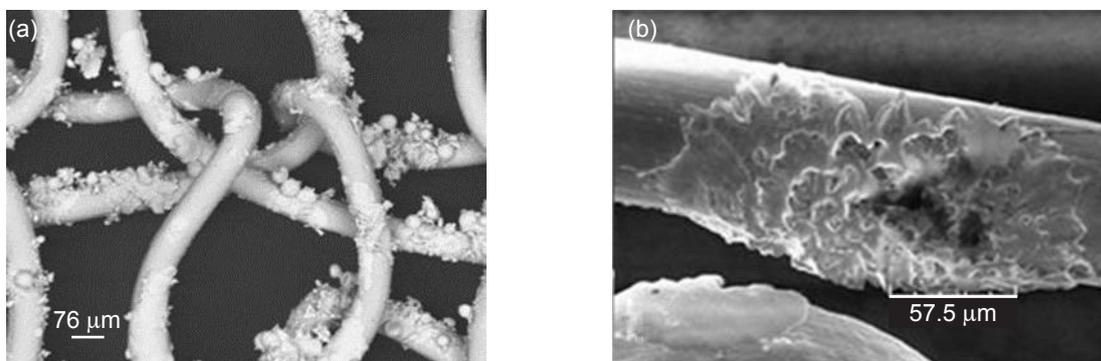
Fig. 10. Scanning electron microscopy (SEM) images of the ACT™ coated gauze
