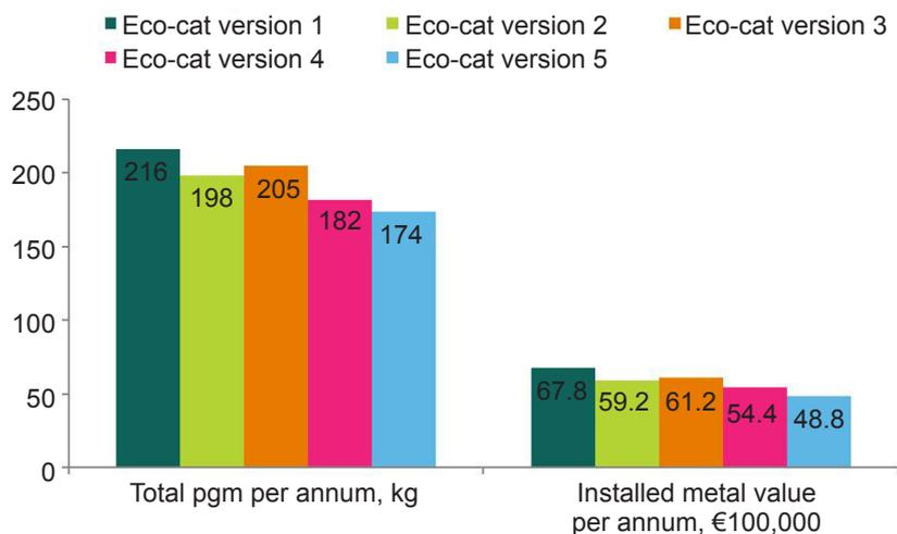
Fig. 5. The pgm content and value in developments of Eco-Cat™ packs
