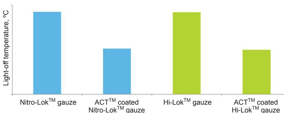
Fig. 9. Graph demonstrating a reduction in light-off temperature with ACT™ coatings
