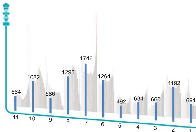
Fig. 1. Tracer Production Log™ (TPL) of stage contribution. The bar chart is a representation of the individual stage comparable production, using arbitrary axes. The dark blue bar is to represent the total stage output over the time frame indicated by the multiple faded bars. The multiple faded bars represent individual sample comparisons of production per stage
