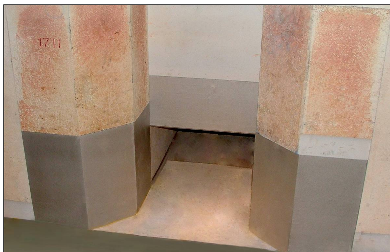
Fig. 4. A furnace throat, ACT ® coated with a platinum-rhodium alloy. The throat is constructed from fused cast ceramics (in this case ER 1711 RT (40% ZrO 2 ) from Saint-Gobain SEFPRO): the surface of these materials is laser drilled prior to coating to ensure a strong, uniform adhesion of the coating
