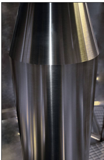
Fig. 3. A Danner sleeve for the manufacture of glass tubing for pharmaceutical components is ACT ® coated with platinum and then fully polished
