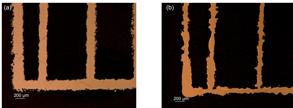
Fig. 3. Cross-section of walls of model part produced by selective laser melting (3D printing) using 62.5 W laser power and  $0.33 \text{ m s}^{-1}$  scanning speed in: (a) platinum and (b) 18 carat gold (Courtesy of Damiano Zito (ProGold SpA, Italy))
