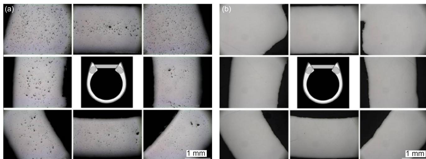
Fig. 1. Test cast ring in Pt-5Ru (centre) showing microsections of castings: (a) as-cast with double sprue, showing substantial shrinkage porosity; (b) after HIP showing removal of porosity (Courtesy of Teresa Fryé (TechForm Advanced Casting Technology, USA))
