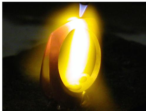
Fig. 1 Working a palladium alloy ring (courtesy of Mann Design Group)
