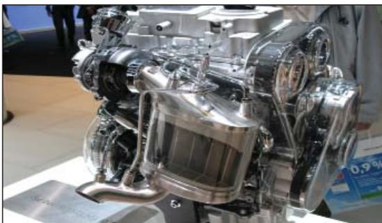
Fig. 1. A compact catalysed particulate matter filter mounted directly on the turbocharger of a small diesel engine (Image copyright Martyn V. Twigg)
