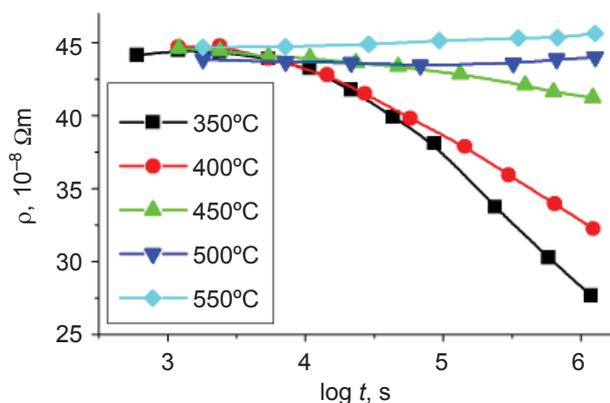
Fig. 5. The dependence of the electrical resistivity of Cu-55Pd on the holding time at different temperatures
