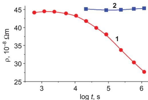
Fig. 2. The dependence of resistivity on the holding time at 350°C of Cu-55Pd alloy in different initial states: after SPD (curve 1) and after quenching from 750°C (curve 2)
