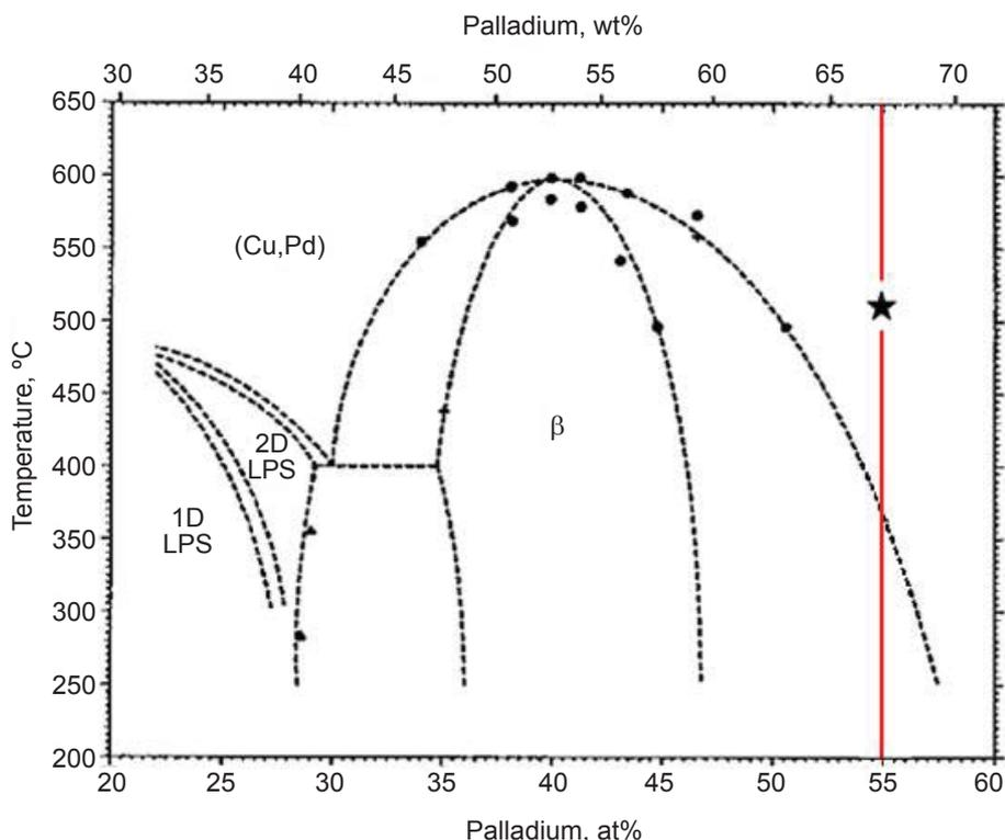
Fig. 1. Portion of the phase diagram of the Cu-Pd system (1). The vertical line denotes the alloy composition studied. The sign “★” marks the temperature boundary of the  $A1 \rightarrow (A1+B2)$  transformation of the Cu-55Pd alloy that was determined in this study
