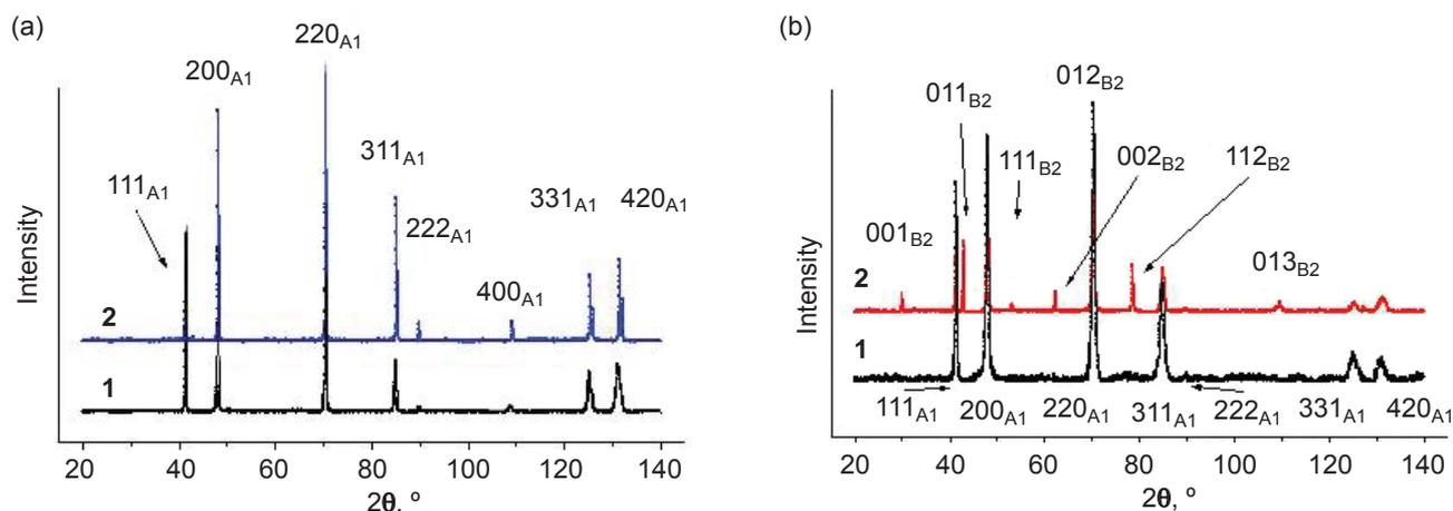
Fig. 3. XRD patterns from the alloy Cu-55Pd in the initial state (pattern 1) and after annealing (pattern 2) at a temperature of 350°C for 306 h (2): (a) quenched; (b) subjected to SPD
