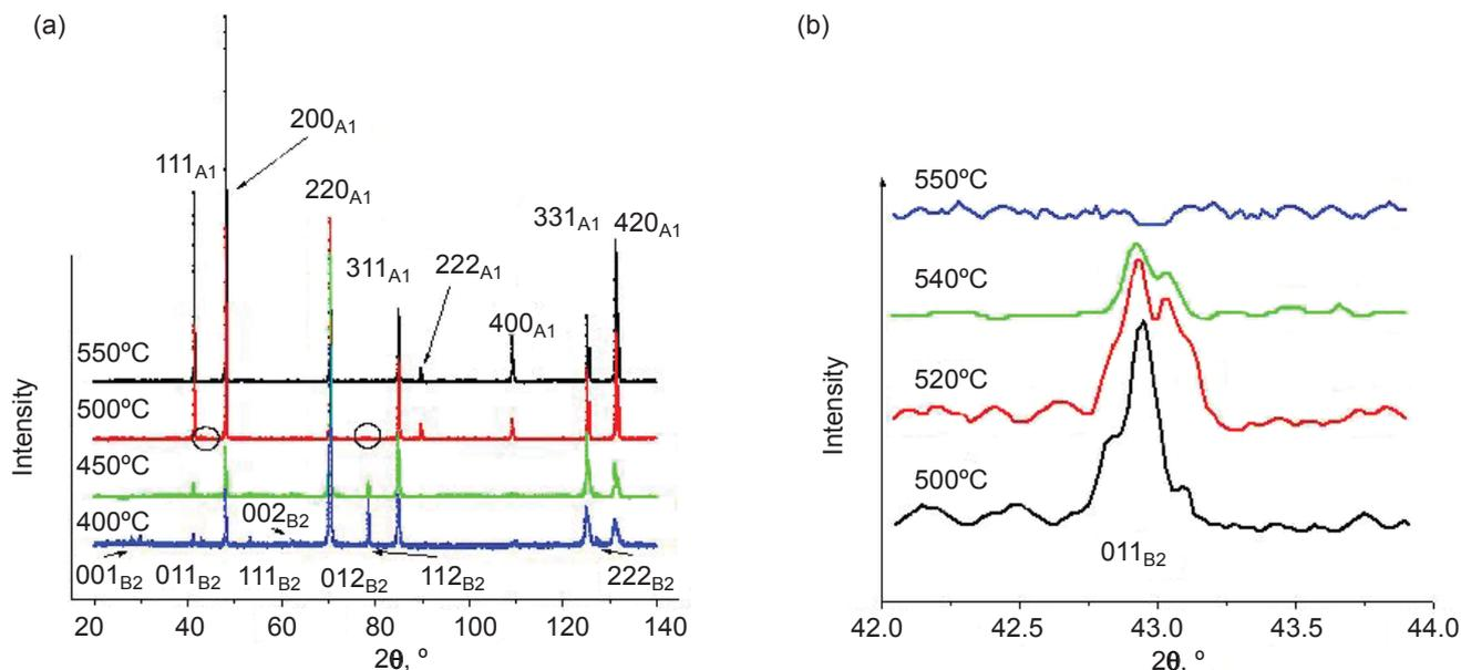
Fig. 4. XRD patterns from the studied alloy subjected to SPD and subsequent holding at various temperatures for 336 h: (a) 400°C –550°C; (b) 500°C –550°C ( $2\theta = 42^\circ - 44^\circ$ )
