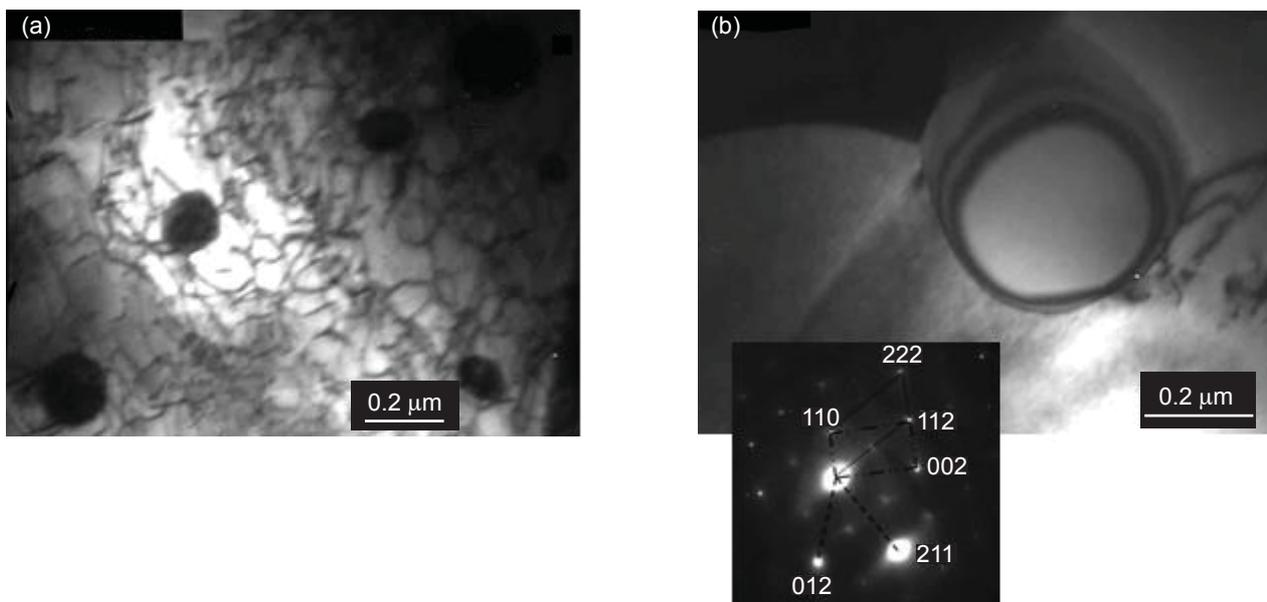
Fig. 7. The bright-field images of Cu-55Pd alloy after SPD to  $\epsilon \approx 3.8$  (the plate 0.2 μm thickness) and annealing at 500 °C for 336 h: (a) a typical microstructure; (b) the microstructure containing B2-phase precipitation (the inset shows a selected area diffraction pattern of the precipitation)
