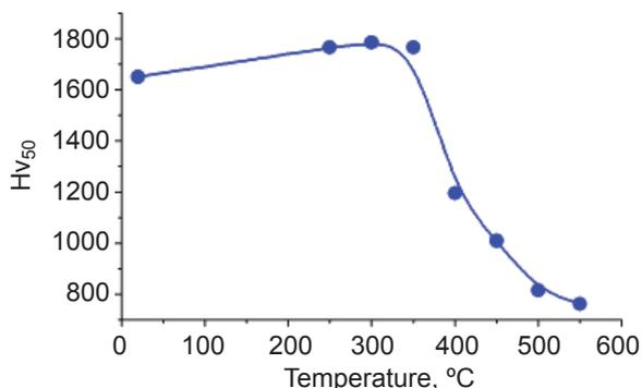
Fig. 6. The dependence of microhardness on the holding temperature for 336 h of samples of Cu-55Pd alloy subjected to SPD
