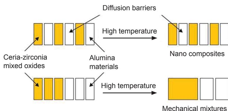
Fig. 2. Schematic illustration of Al<sub>2</sub>O<sub>3</sub> particles as diffusion barriers in CeO<sub>2</sub>-ZrO<sub>2</sub> mixed oxides to improve washcoat thermal stability
