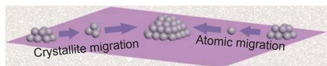
Fig. 3. Two conceptual models for sintering of active precious metal particles
