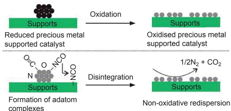
Fig. 5. A schematic representation of redispersion for active precious metals
