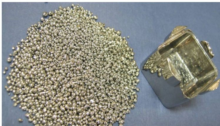
Fig. 1 Thermoplastic forming of 850 platinum bulk metallic glass (BMG) from BMG pellets (Courtesy of B. Lohwongwatana)
