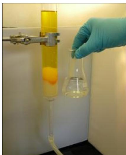
Fig. 2. Smopex<sup>®</sup> test column, showing the effective recovery of platinum from a solution of  $\sim 500 \text{ mg l}^{-1}$  chloroplatinic acid in aqueous, dilute hydrochloric acid
