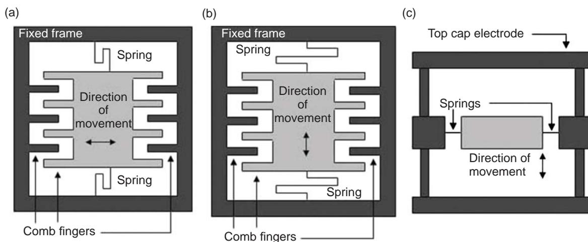
Fig. 1. Three types of electrostatic energy harvester: (a) in-plane overlap varying; (b) in-plane gap closing; (c) out-of-plane gap closing (Reproduced by permission of The Royal Society of Chemistry)
