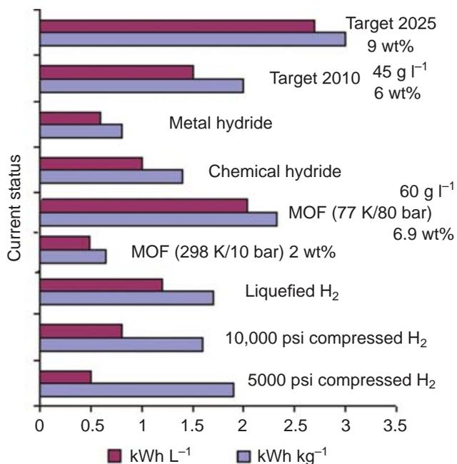
Fig. 2. The current status of today’s hydrogen storage technologies in volumetric and gravimetric terms (Reproduced by permission of The Royal Society of Chemistry)
