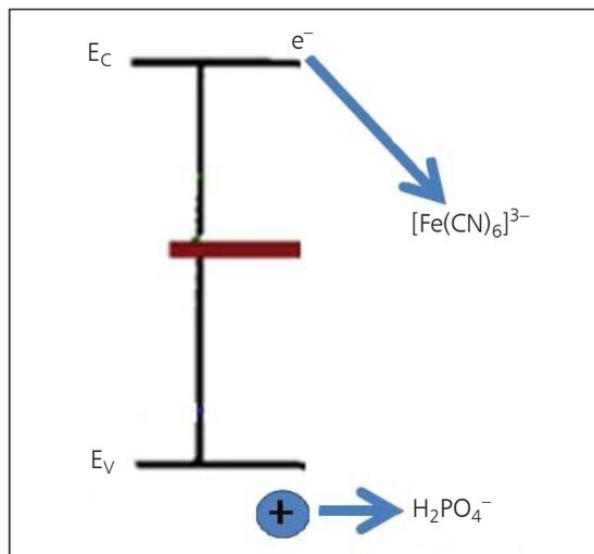
Fig. 6. Energy map for conduction ( $E_C$ ) and valence ( $E_V$ ) bands relative to the  $[\text{Fe}(\text{CN})_6]^{3-}$  energy band
