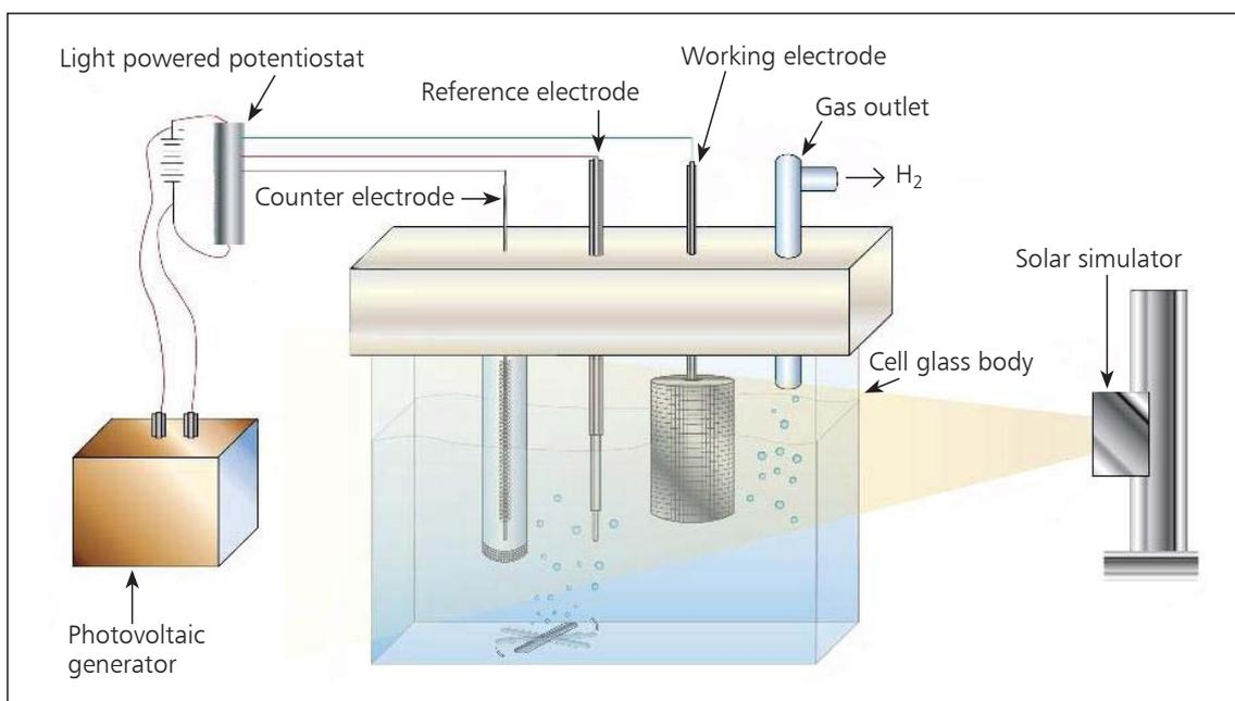
Fig. 2. Diagram of a photolysis cell
