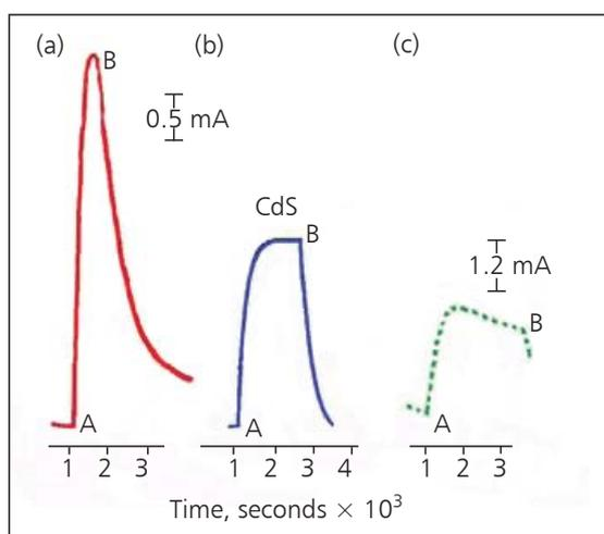
**Fig. 4.** Photoelectrochemical response of the platinum working electrode during the photolysis of 20 mM  $K_4[Fe(CN)_6]$  in 0.2 M phosphate buffer at pH 6: (a) homogeneous solution only; (b) in presence of CdS colloidal nanoparticles; (c) in presence of  $TiO_2/V_2O_5$  (1:1) colloidal nanoparticles. Points A and B refer to illumination and dark, respectively
