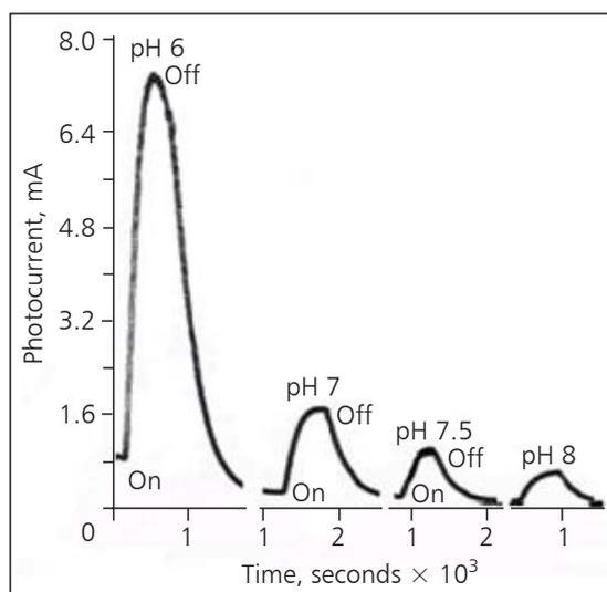
Fig. 3. Effect of pH on the reduction current recorded by the Pt working electrode
