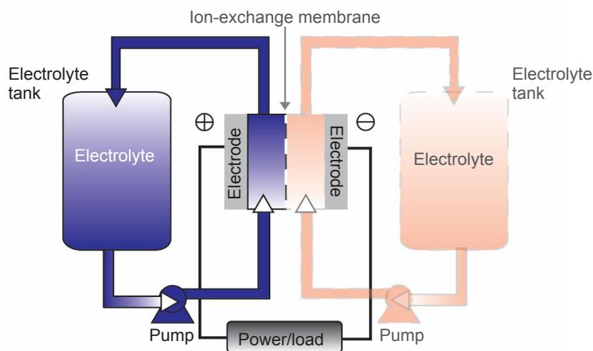
Fig. 3. A conventional RFB has two electrolytes, separated by an ion-exchange membrane and requiring duplicate storage and flow mechanisms. A membrane-free system uses a single electrolyte for reactions at both electrodes, eliminating a large proportion of the components (indicated by the faded out sections) (Reproduced with permission)
