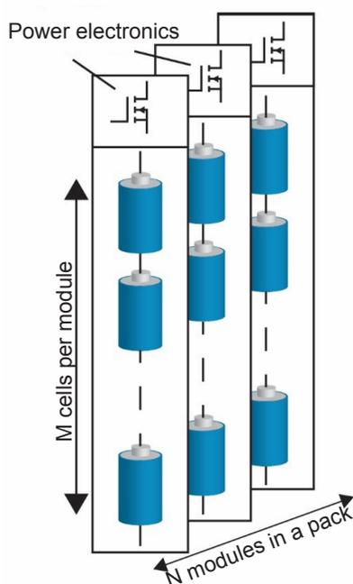
Fig. 1. The cells in a battery pack can be divided up into  $N$  modules, with each module of  $M$  cells controlled by power electronics (Reproduced with permission)
