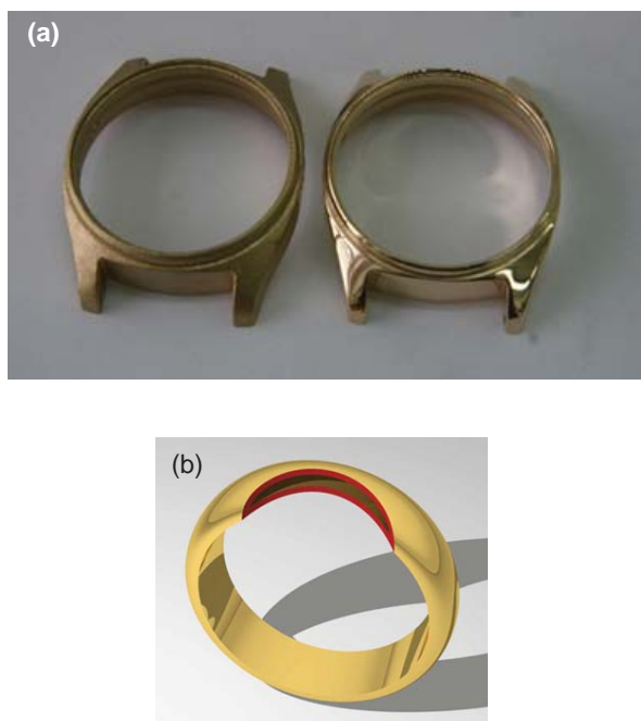
Fig. 11. Volume without mass (right and wrong): (a) watch bezel; (b) CAD image of a hollow wedding band
