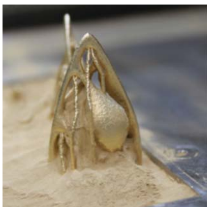
Fig. 6. The Ojo emerges from the powder bed
