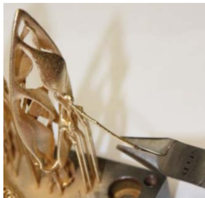
Fig. 7. Support removal from the Ojo
