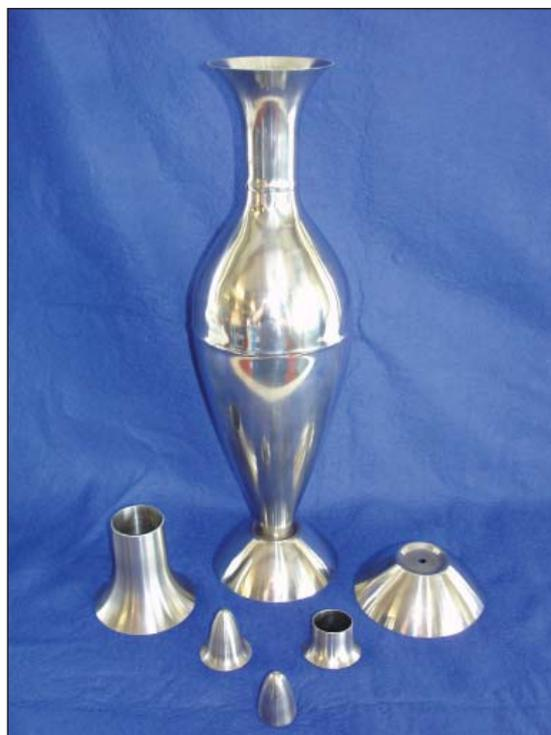
Fig. 1. Palladium jug: tungsten inert gas (TIG)-welded body and other spun parts, spun by Johnson Matthey
