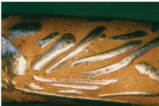
Fig. 6. Platinum wire studs and nuggets in red gold powder, pressed and sintered
