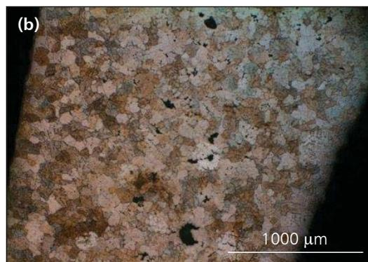
Fig. 3(a). Grain structure of as-cast conventional Pt-5 wt% Co alloy; (b) refined grain structure of '95-Pt-Co+' alloy hardened with gallium (Courtesy of Teresa Fryé (TechForm Advanced Casting Technology, USA))
