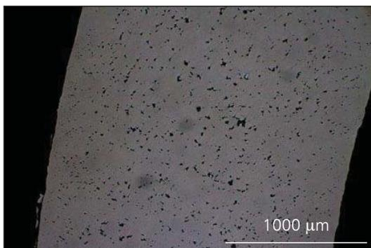
Fig. 2. Microstructure of as-cast coupon of Pt-5 wt% Ru alloy showing porosity distributed throughout section (Courtesy of Teresa Fryé (TechForm Advanced Casting Technology, USA))
