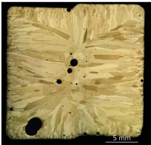
Fig. 4. Transverse section of Pt-5 wt% Cu alloy as cast bar (hardness HV 130). Columnar grains and porosity are visible (Courtesy of Paolo Battaini (8853 SpA, Italy))
