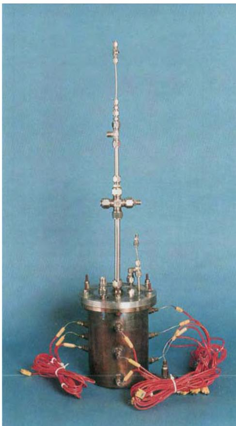
Fig. 1 A prototype of the HotSpot™ reactor for hydrogen generation (4)
