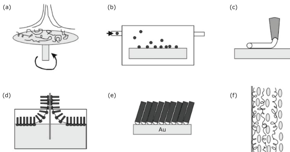
Fig. 2. Various types of technologically important thin organic films: (a) spin-coated films; (b) organic vapour-phase deposited films; (c) inkjet-printed films; (d) Langmuir-Blodgett films; (e) self-assembled monolayers; and (f) layer-by-layer films. Copyright Wiley-VCH Verlag GmbH & Co KGaA. Reproduced with permission
