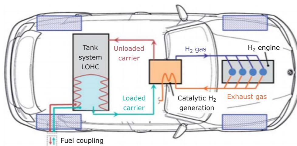
Fig. 5. Schematic representation of the LOHC technology within a motor vehicle. Republished with permission of The Royal Society of Chemistry, from (50); permission conveyed through Copyright Clearance Center, Inc
