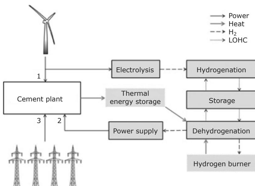
Fig. 3. Schematic representation of the coupling of a cement plant to a LOHC system. Reproduced from (38), Copyright © 2016 WILEY-VCH Verlag GmbH & Co. KGaA, Weinheim
