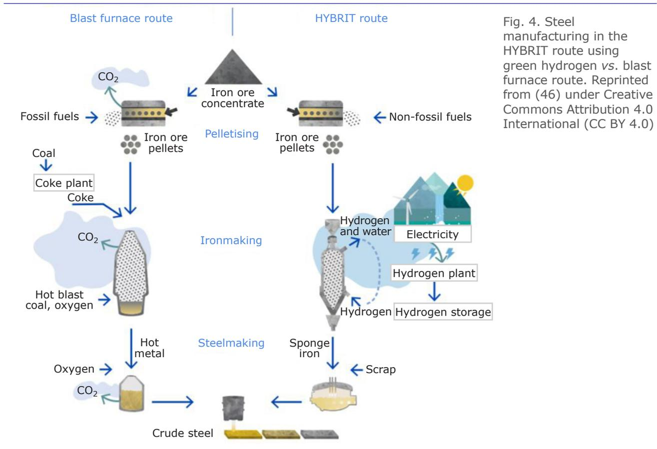
Fig. 4. Steel manufacturing in the HYBRIT route using green hydrogen vs. blast furnace route. Reprinted from (46) under Creative Commons Attribution 4.0 International (CC BY 4.0)
