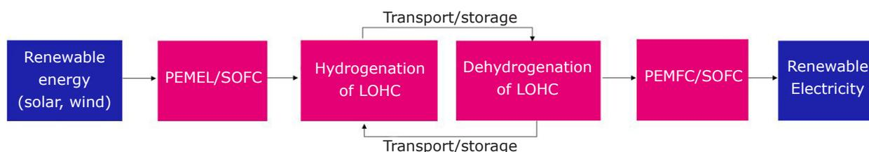
Fig. 1. Schematic representation of the integration of fuel cells into LOHC technology (25)
