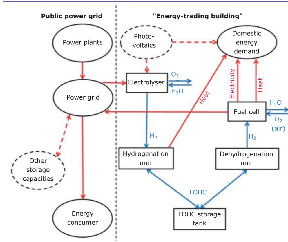
Fig. 2. Concept of integrating LOHC and fuel cell technologies to provide domestic energy. Republished with permission of The Royal Society of Chemistry, from (34); permission conveyed through Copyright Clearance Center, Inc
