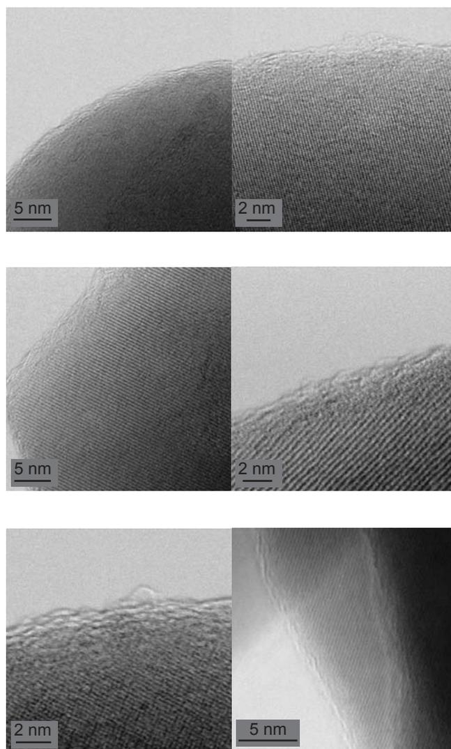
Fig. 2. TEM images of carbon coated  $\text{LiFePO}_4$
