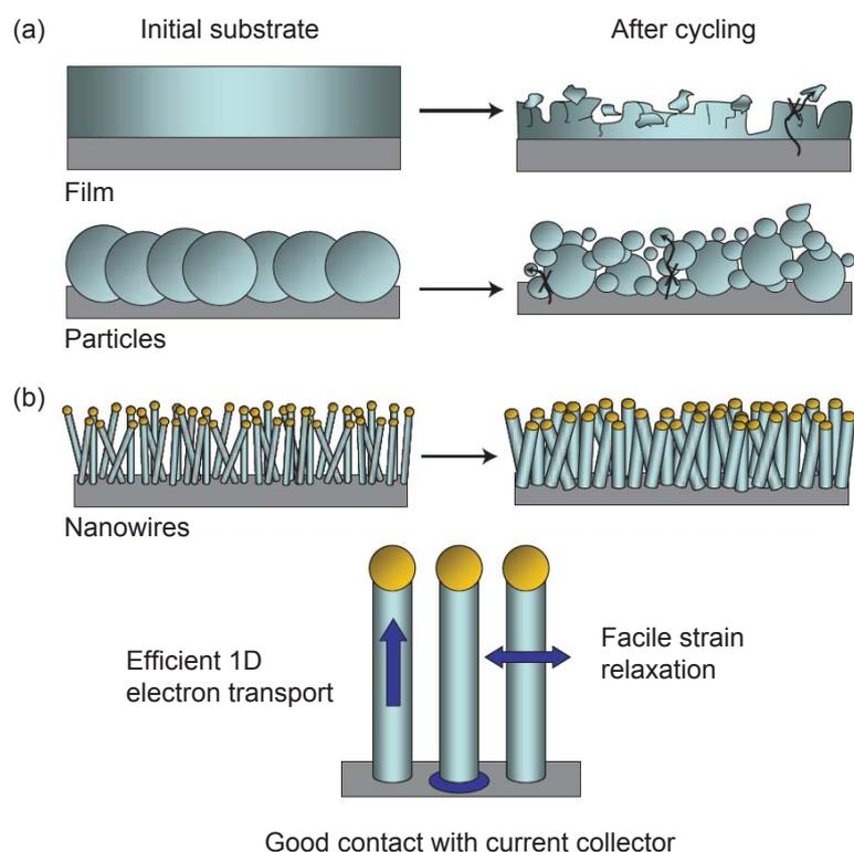
Fig. 1. Schematic of morphological changes that occur in Si during electrochemical cycling. (Reproduced with permission from (1). Copyright (2008) Nature Publishing Group)
