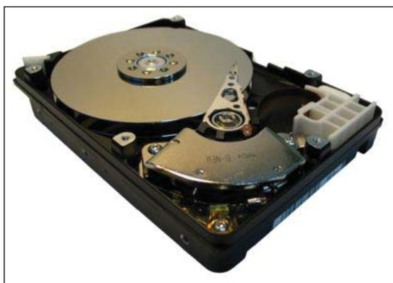
*Fig. 1. Hard disk drive with cover removed, showing the pgm-containing disk in which information is stored*
