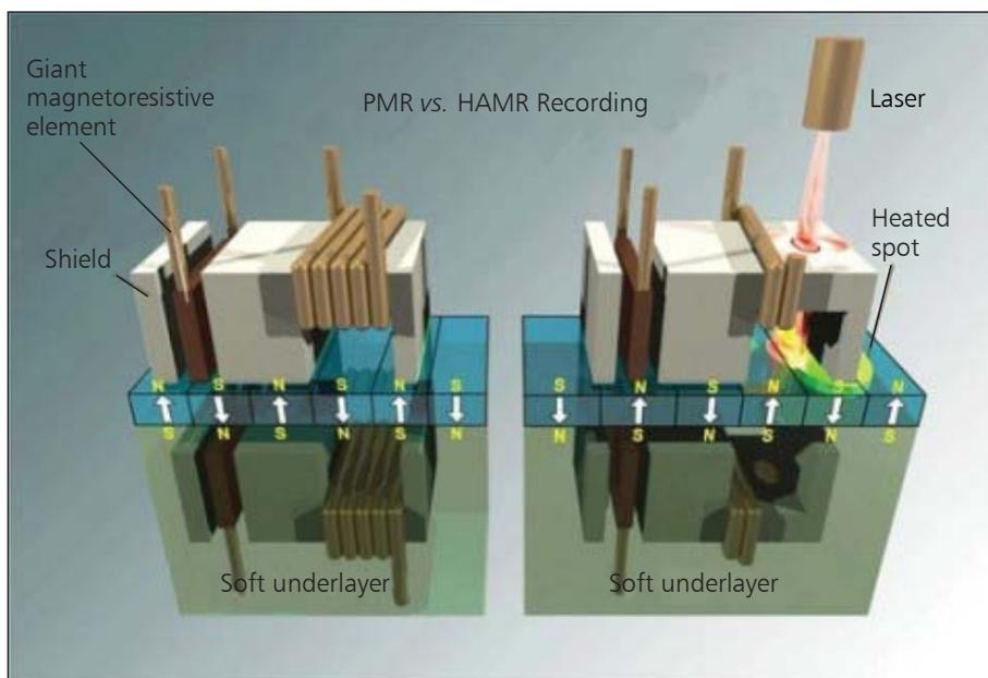
Fig. 3. Schematic image showing the difference between HAMR and PMR technology (Courtesy of Seagate Technology)
