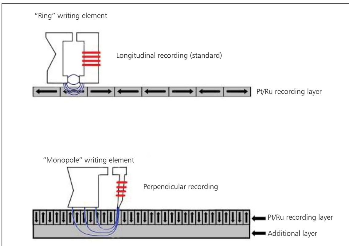
Fig. 2. Basic concept of longitudinal magnetic recording (LMR) and perpendicular magnetic recording (PMR) designs
