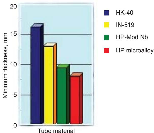
Fig. 5. Comparison of HK-40 15.5 mm, HP-modified Nb 10 mm and HP microalloy 8 mm tube wall thickness (7)
