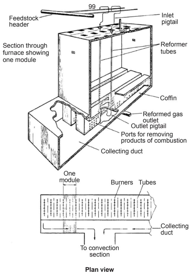
Fig. 4. Modular top fired reformer design by Davy Powergas Ltd in 1973 (6)
