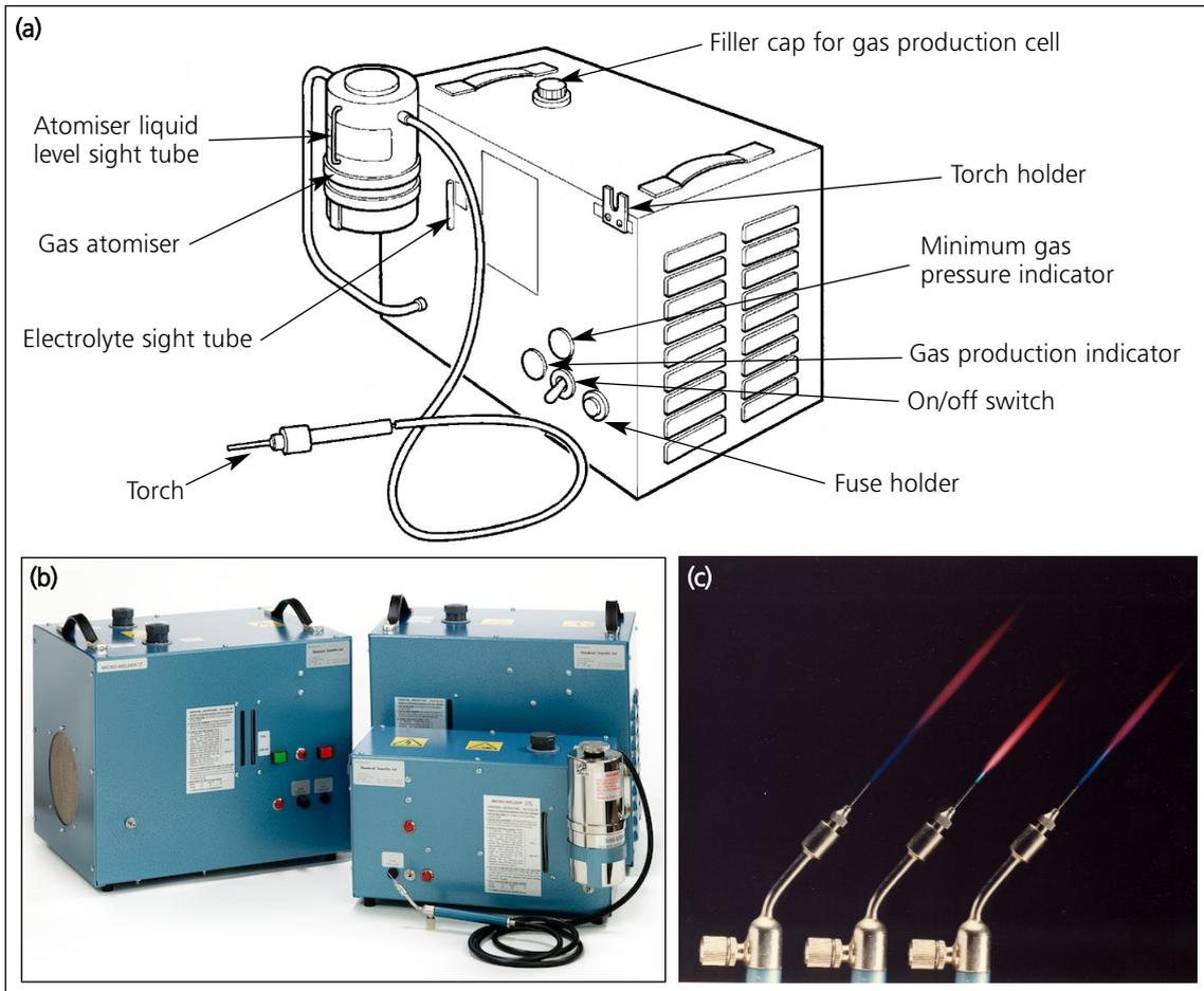
Fig. 1. (a) Schematic diagram of a microwelder (3); (b) A range of microwelders; (c) Microwelder torch flames showing boosted luminosity (Figures 1(b) and 1(c) courtesy of Sherwood Scientific Ltd (4) and A G Thomas (Bradford) Ltd (5))
