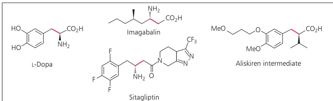
Fig. 8. Some products of industrial rhodium-catalysed asymmetric hydrogenation processes (hydrogenated bonds in bold red)
